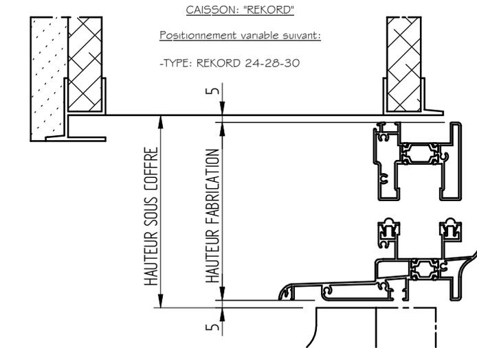
HT FABRICATION = HT SOUS COFFRE - 10
